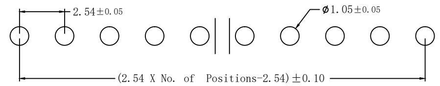
Recommended PCB Layout
